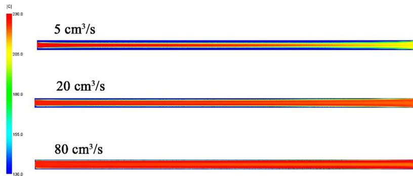
Fig. 7. The temperature distribution of the injection molded specimens at various flow rates.
